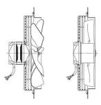
Axial fan with external electromotor(Right) with Internal electromotor (Left)
